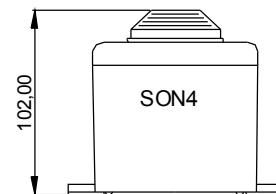
SON4 24vdc unit is CPD Compliant. EN54-3 Type B IP55. Beacon is not compliant.
